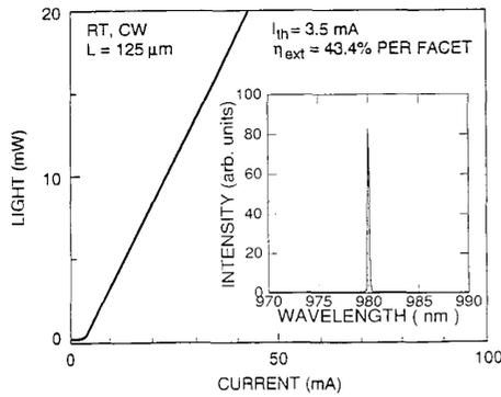
Fig. 2. A typical continuous-wave light-current characteristics of a 3- $\mu\text{m}$ -wide and 125- $\mu\text{m}$ -long ridge waveguide laser at room temperature with cleaved facets. A low threshold current of 3.5 mA with a high differential quantum efficiency of 87% is obtained. The inset shows the lasing spectra at 980 nm with the laser biased at  $1.6I_{\text{th}}$ .
