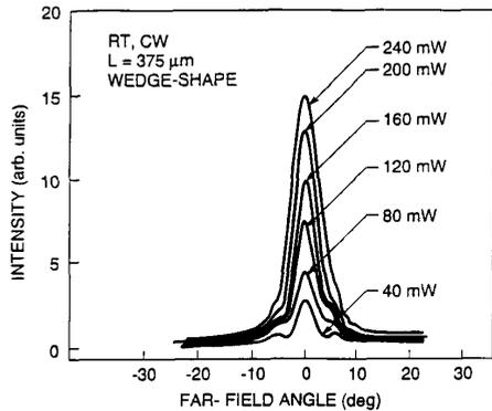
Fig. 5. The far-field radiation patterns measured from a 375- $\mu\text{m}$ -long wedge-shaped ridge-waveguide laser showing the dominating single-lobe operation up to 240 mW of continuous-wave output power. A maximum output power of 310 mW was obtained from this AR/HR-coated laser before the facet was damaged.
