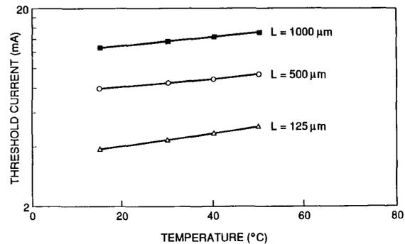
Fig. 4. The temperature dependence of the threshold currents of as-cleaved 3- $\mu\text{m}$ -wide AR/HR-coated ridge lasers from 15 to 50°C. A high characteristic temperature of 220 K is derived for lasers with 500  $\mu\text{m}$  and 1 mm cavity lengths.
