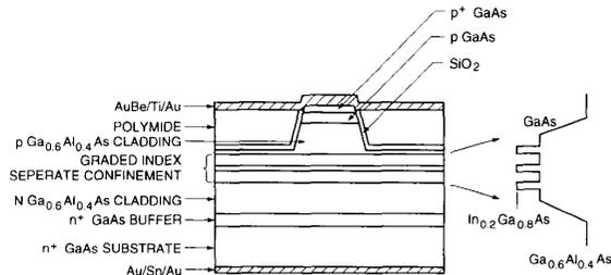
Fig. 1. The layer structure of the graded-index separate-confinement (GRIN SCH) laser grown by organometallic vapor phase epitaxy.
